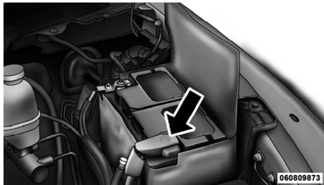
Positive Battery Post
